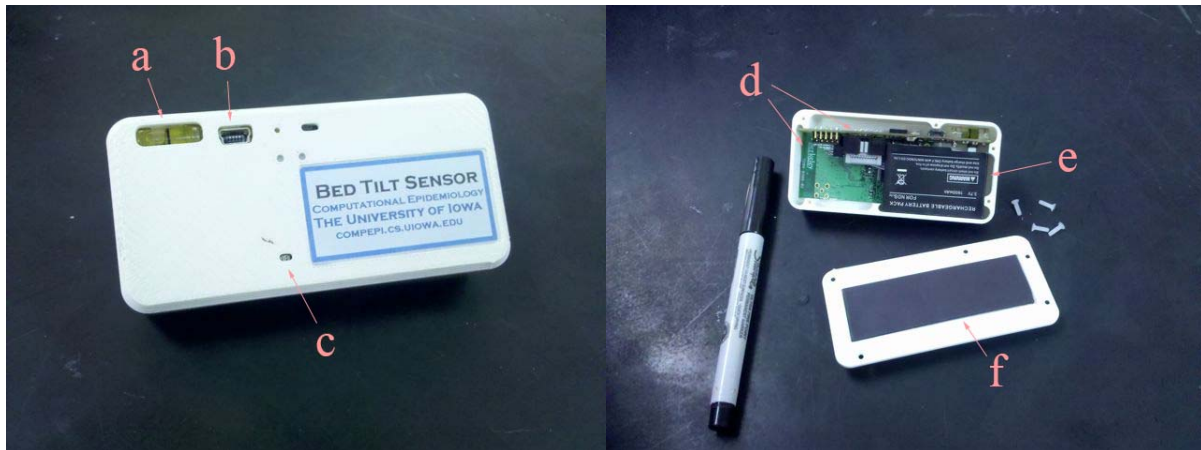
Figure 1: To the left, a prototype of the bed angle monitor with: a) bubble level indicator, b) USB port, and c) LED indicators. To the right, the inside of the device revealing: d) two circuit boards, e) a rechargeable battery, and f) the magnet on the back cover. 47
