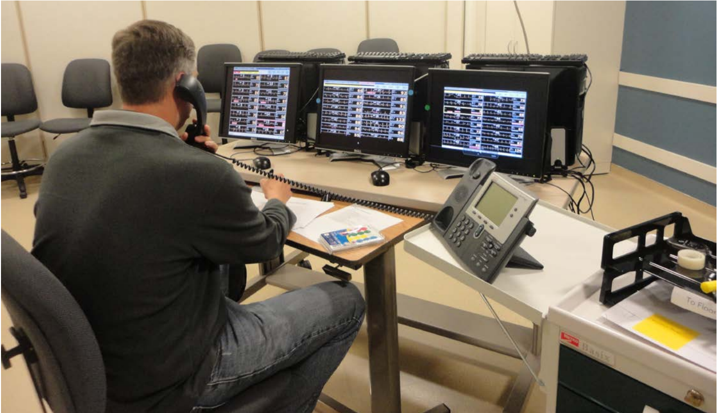
Figure 2. Experimental setup for 48 patients. One patient is simulated with a VF arrhythmia (on the left display). ECGs for the remaining 47 patients are real (pre-recorded).
